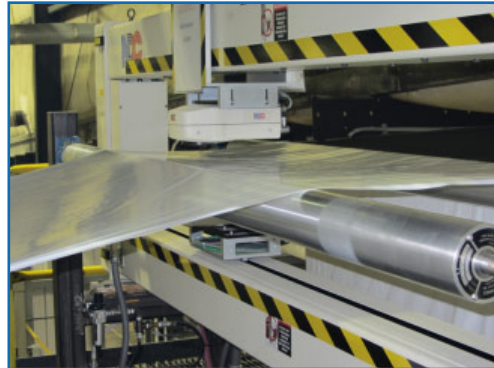
NDC's FG710S infrared sensor scanning double layflat blown film
