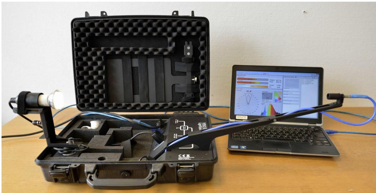
**Figure 1 – Photo of the portable spectrometer system in operation with a laptop computer controlling the measurement.**
