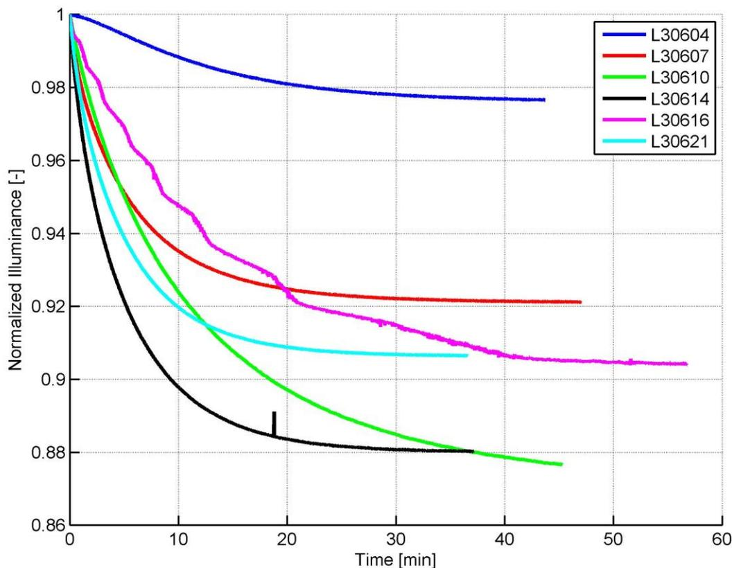
**Figure 3 – Measured normalized illuminance as a function of time after the DUT is turned on.**
