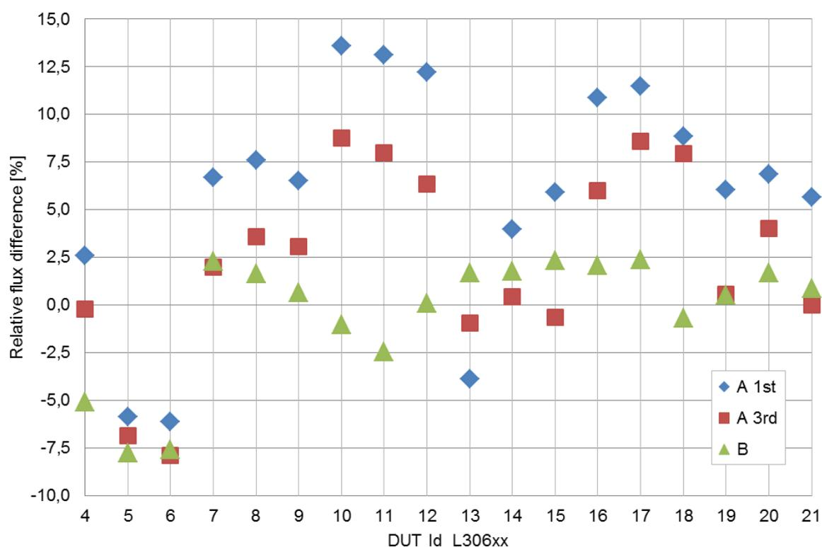
**Figure 2 – Relative differences of total luminous flux for DUTs for the three different measurements.**
